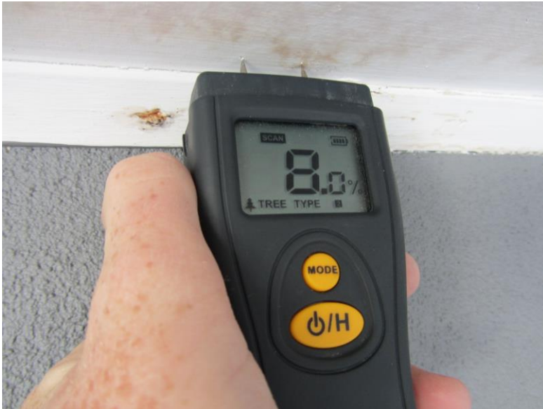
Photo 1. Shows a moisture level reading prior to testing beginning.
